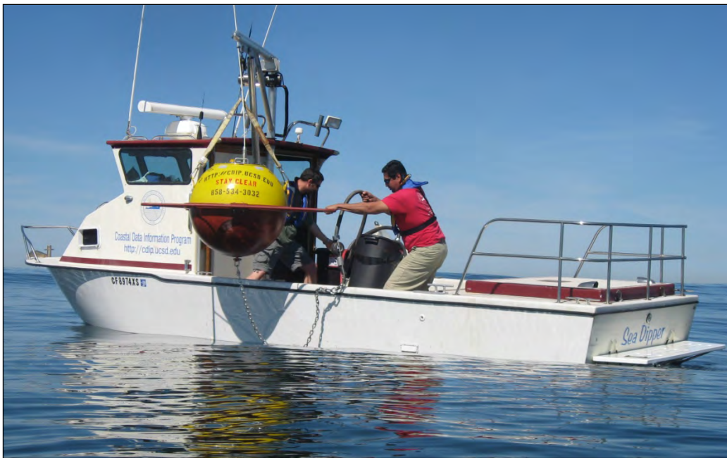
Figure 4: Example of CDIP wave buoy being deployed.
