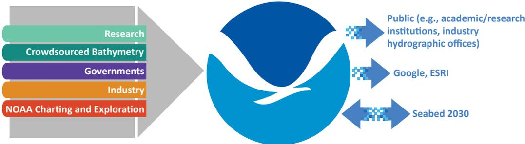
Crowdsourced bathymetry is the collection of depth measurements from vessels with standard navigation instruments during routine maritime operations. It is a powerful source of information that helps to fill gaps where data is sparse, especially in places where government survey vessels do not have the resources to go in the next ten years.
