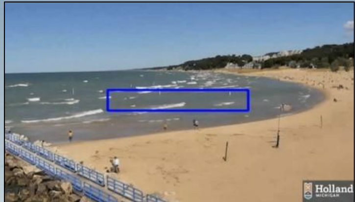
A still image from the high-resolution WebCOOS webcam located at Holland, MI. The video shows the detection of a rip current (blue box) using Artificial Intelligence at Holland Beach, MI.
