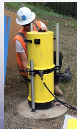
Absolute gravity observation on passive mark.
