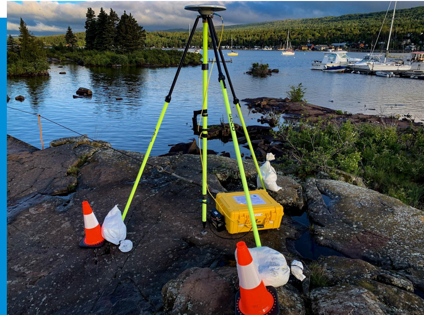
Image: GNSS occupation of bench mark in Grand Marais, MN; Photo credit: Gavin
