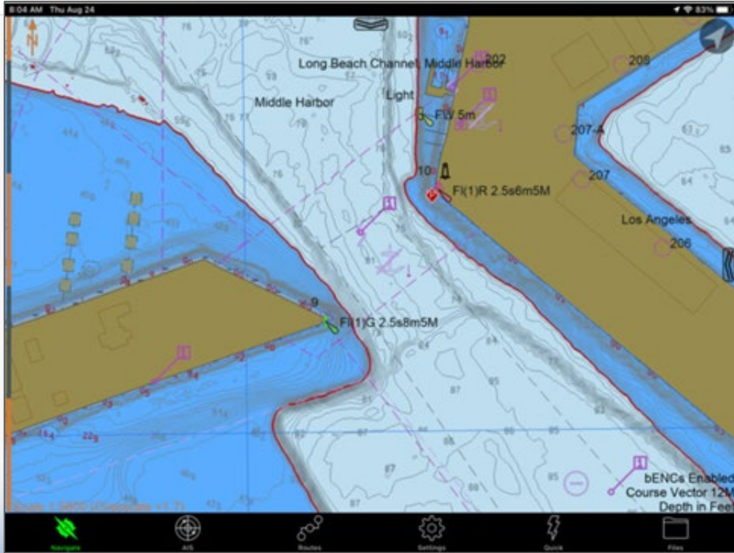
Jacobsen Pilot's portable pilot unit screen using the navigation system SEAIq Pilot, and S-102 data to draw custom safety contours. Credit: Jacobsen Pilot Service.
