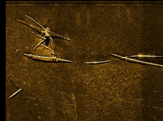
Exposed Pipelines (Mosaicked Surface)
