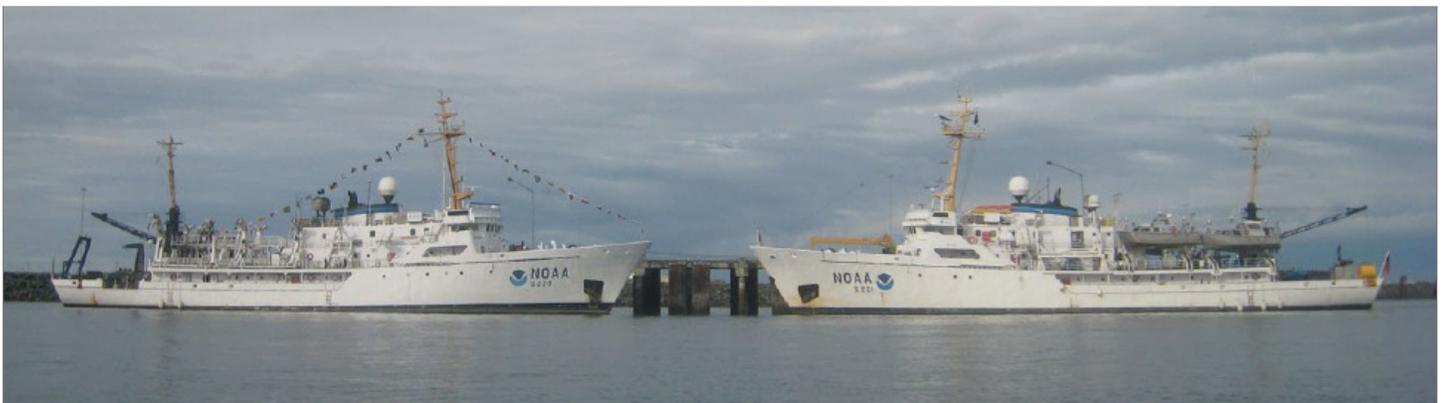
*NOAA ships Rainier and Fairweather were built in 1968 with an original design life of 30 years. Each ship carries five survey launches. Dedicated ships carrying multiple survey launches are one of the most efficient and cost-effective ways to conduct hydrographic surveys. Both vessels still conduct annual surveys in challenging Alaskan and Arctic waters.*
