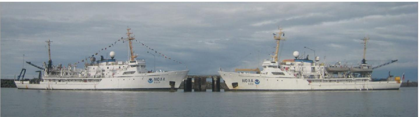
*NOAA ships Rainier and Fairweather were built in 1968 with an original design life of 30 years. Each ship carries five survey launches. Dedicated ships carrying multiple survey launches are one of the most efficient and cost-effective ways to conduct hydrographic surveys. Both vessels still conduct annual surveys in challenging Alaskan and Arctic waters.*
