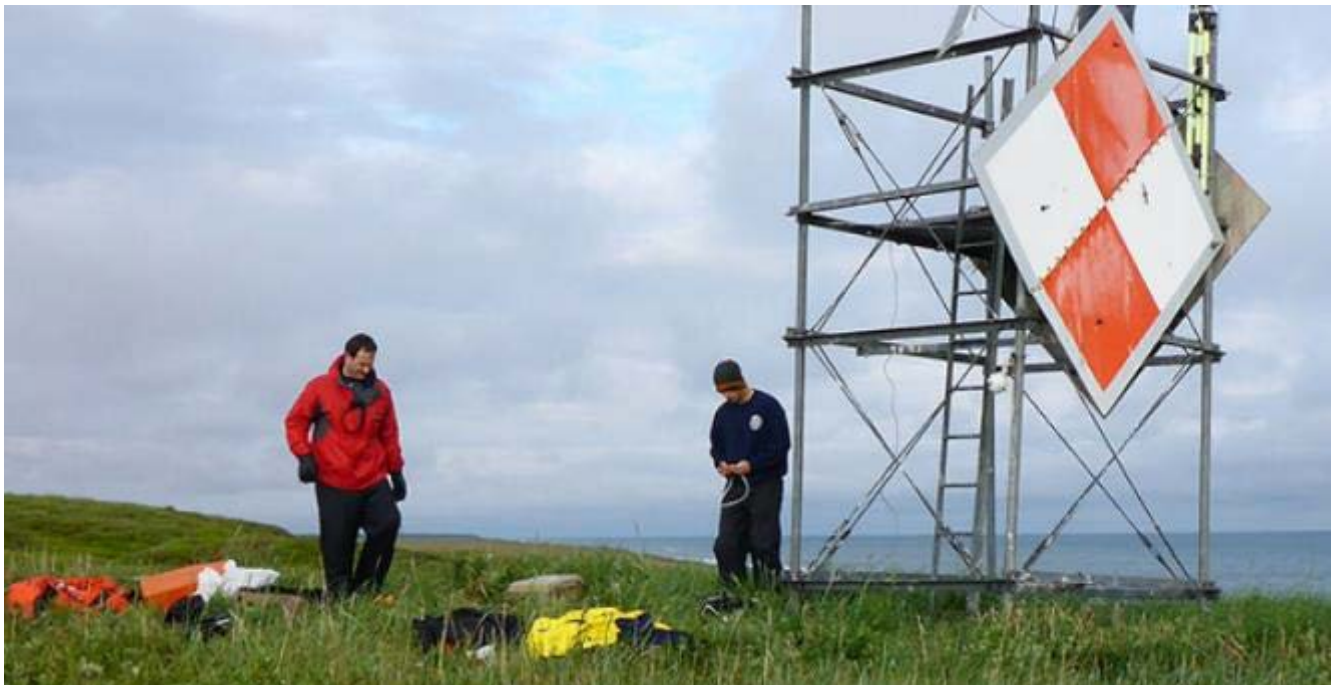
Ensign Christopher Wood, Ensign Samuel (Woodrow) McKay, and Ensign Dylan Kosten establish a horizontal control station on a U.S. Coast Guard day marker in the Arctic.
