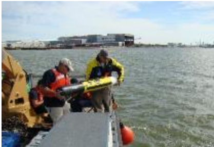
Small AUV deployed for post-storm survey in Galveston Harbor.
