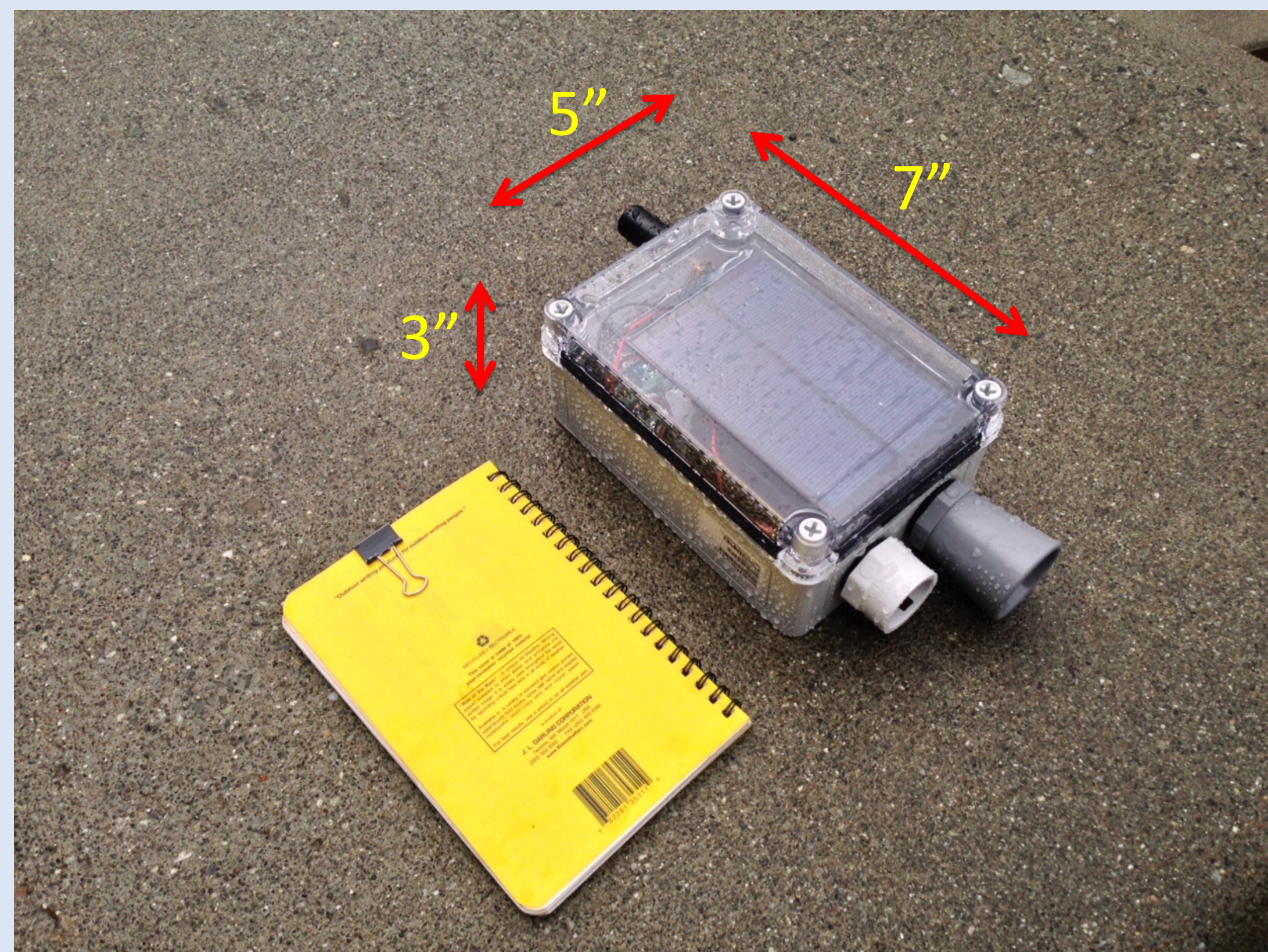
Figure 1. The iGage is a compact, low cost acoustic sensor used by the NWS to measure river stages, coastal water levels and snow depths.
