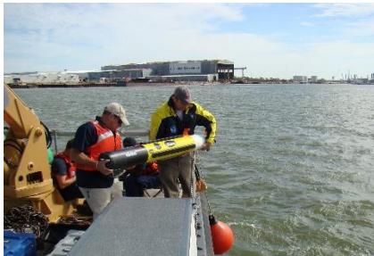
Small AUV deployed for post-storm survey in Galveston Harbor.
