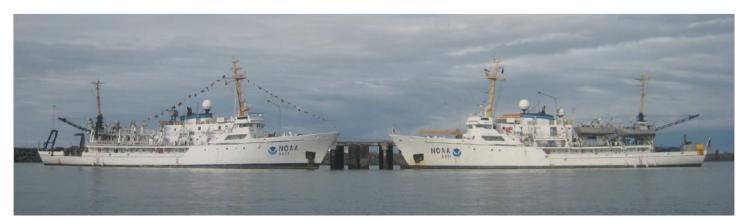
NOAA ships Rainier and Fairweather were built in 1968 with an original design life of 30 years. Each ship carries five survey launches. Dedicated ships carrying multiple survey launches are one of the most efficient and cost-effective ways to conduct hydrographic surveys. Both vessels still conduct annual surveys in challenging Alaskan and Arctic waters.
