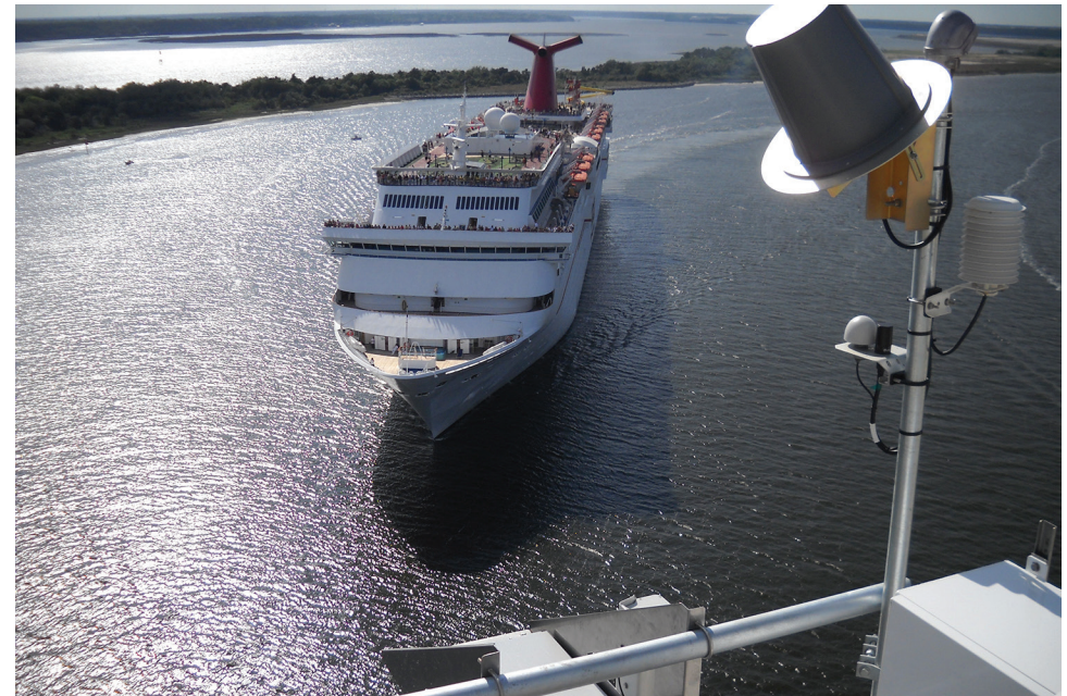
Air gap installation on Dames Point Bridge in Jacksonville, Florida. Credit: Steve O'Malley, Ocean Tech Services, LLC
