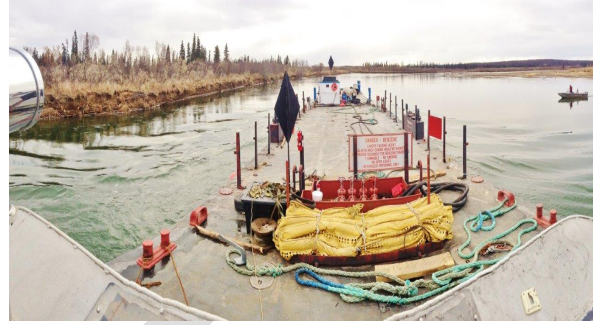
Figure 3. This shows a tug barge going up an Alaska inlet, preceded by the sounding skiff in the distance that determines safe depths for passage. They would be much more efficient with GPS/GNSS and known depth data.
