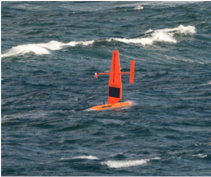
Figure 16. Although the Saildrones operating in the Arctic are equipped with single-beam sonar, options are available also for multi-beam sonar.
