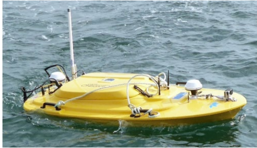
Figure 14. The Z-boat, with multibeam sonar, is one of many options to choose from on surveying shallow waters for NOAA's coastal mapping program and to fill voids from topobathy lidar where waters are too turbid for full bottom coverage.
