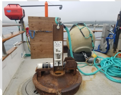
Figure 9. Non-vented pressure, conductivity and temperature sensors secured to an oceanographic anchor prior to deployment south of the Alaska Peninsula.
