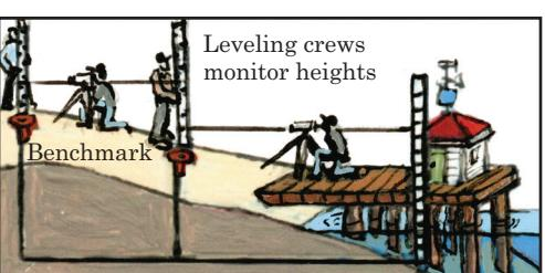
Cartographers use the information collected from tide gauges and benchmarks to create tidal datums. They record these different water-level averages on the charts. To clear bridges and overhead cables, mariners refer to Mean High Water (MHW). To avoid underwater obstructions mariners, refer to Mean Lower Low Water (MLLW).
