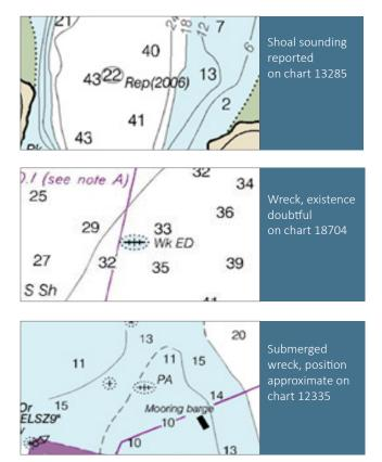
Figure 4. Examples of cartographic representations of unverified hazards to navigation.
