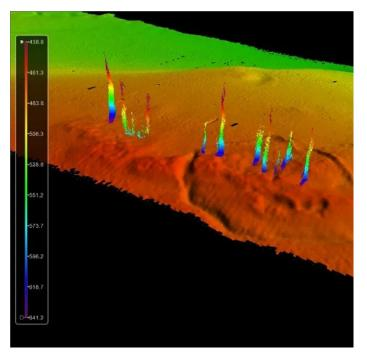
Figure 6. Perspective view of methane gas seeps overlaid on multibeam bathymetry acquired during the Cascadia Margin collaborative seafloor mapping project.
