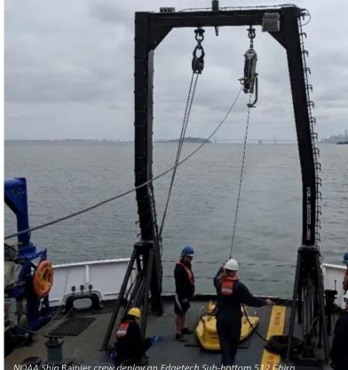
NOAA Ship Rainier crew deploy an Edgetech Sub-bottom 512 Chirp profiler, one of the pieces of equipment brought by the USGS team during the EXPRESS project offshore of Morro Bay, California. Credit: Dr. Maureen Walton, USGS
