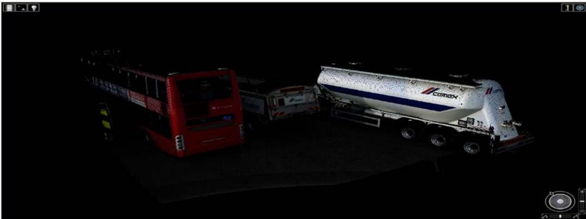
**Figure 4. Sample laser scan point cloud colored by RGB values in BDB 3D View
