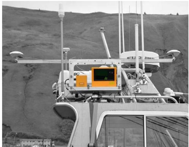
**Figures 1a and 1b. Traditional Shoreline Verification and Vessel-Mounted LiDAR system**
