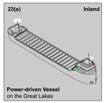
shall be placed as nearly as practicable to the fore and aft centerline of the vessel >>.
