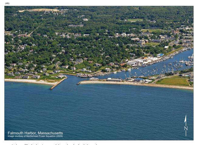
inshore. The harbor is entered through a dredged channel between two jetties; a light marks the end of each jetty.
