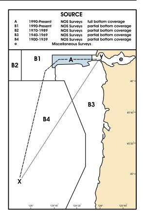
The transit starts again in an area surveyed by NOAA between 1900-1939. The sounding data in this area would have been collected by leadline. Depths between sounding points can only be inferred, and undetected features might still exist between the sounding points in areas of irregular relief — caution should be exercised.
