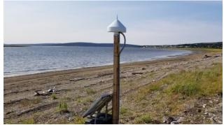
Figure 12. GNSS-Reflectometry water level system installed in Koyuk, AK by JOA Surveys, LLC in support of the NOAA Office of Coast Survey Project OPR-R385-KR-20. TerraSond Ltd. was the prime contractor. Photo courtesy of JOA Surveys.
