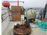
Figure 9. Non-vented pressure, conductivity and temperature sensors secured to an oceanographic anchor prior to deployment south of the Alaska Peninsula.
