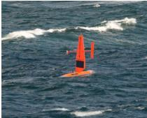
Figure 16. Although the Saildrones operating in the Arctic are equipped with single-beam sonar, options are available also for multi-beam sonar.
