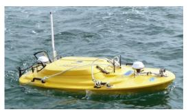
Figure 14. The uncrewed Z-boat, with multibeam sonar, is one option to choose from on surveying shallow waters for NOAA's coastal mapping program and to fill voids from topobathy lidar where waters are too turbid for full bottom coverage.
