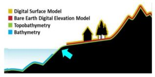
Figure 1. The aqua arrow points to the seamless topobathymetric 3-D surface that includes both underwater bathymetry (depths) and onshore topography (land elevations) with no data gaps at the land/water interface known as the coastal zone or intertidal zone.
