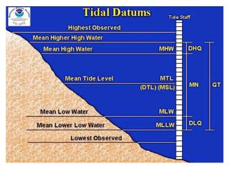
Figure 19. The relationship between various tidal surfaces.
