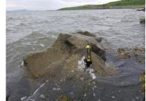
Figure 10. RBR Solo Depth Logger installed at St. Michael, Alaska. This is a non-vented pressure sensor that was intentionally installed above MLLW to measure a portion of the tide range.
